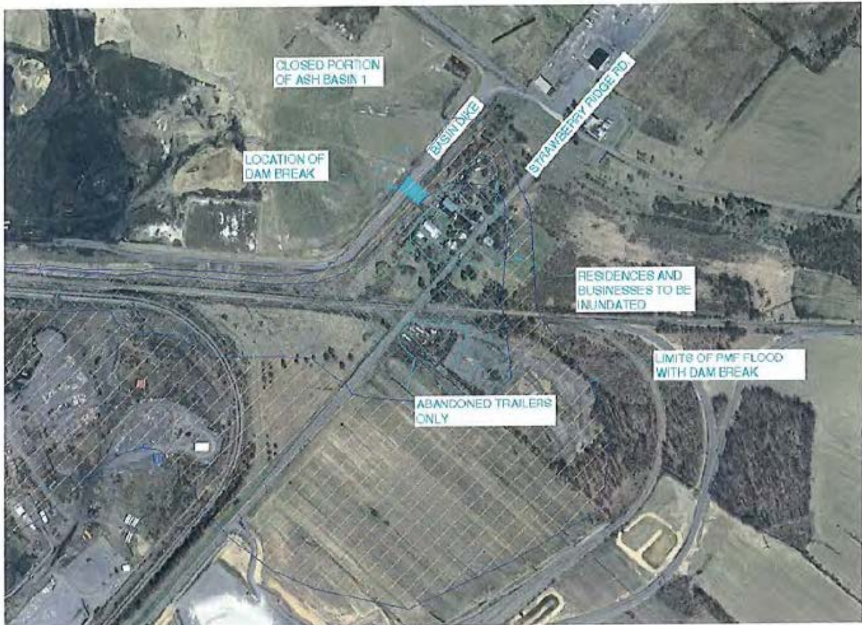
Aerial 3 – Inundation Area – PMF STORM Dam Break at Toe
